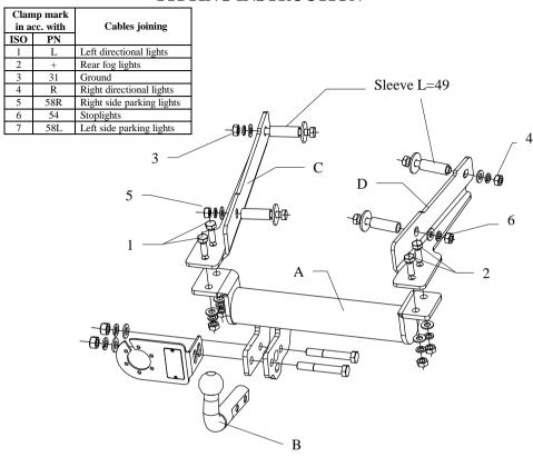
This towbar is designed to assembly in following car:
